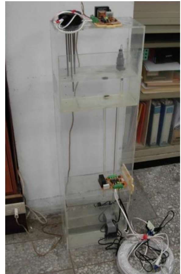
電力線通訊為基礎之液位控制器 A Liquid Level Controller Based on Power Line Communication
