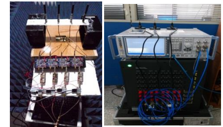
軟體無線定應用於多天線輻射量測 SDR for MIMO OTA testing
